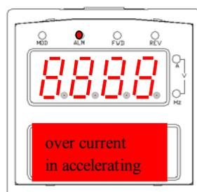
failure alarm display status
