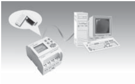
Fig. 4 . 24. FAB Communication Connection Frame
