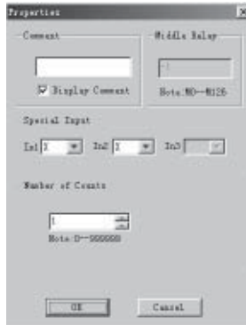
Fig. 3.15 Setting Properties for Blocks with Counters
