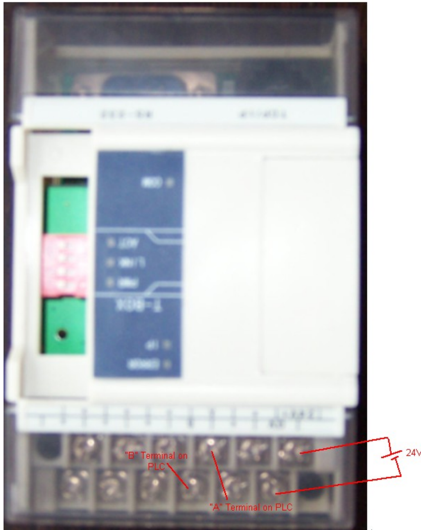
Input power supply: Terminal board 24V DC (24V+, GND)
