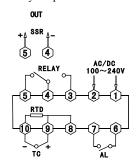
TE7 Power:AC 110/220V±10% Voltage Output:DC 12V 30mA Relay Output:AC 250V 3A
